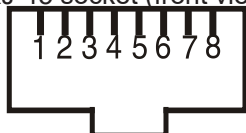
RJ-45 socket (front view):
