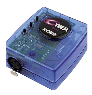
The Cyber Mini is the perfect product for small applications with less than 60 DMX channels. It offers a standalone memory with a maximum of 40 steps (60 channels) as well as 6 (4 + next/previous) ports for dry contacts triggering.
